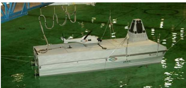
Figure 23 - Model during oblique seakeeping tests
