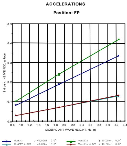
The VERES analysis clearly shows a significant difference between the response of the ModCAT and Vanilla catamaran without motion damping. However, the predicted differences with motion damping are very small.
