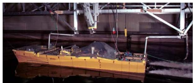
Figure 19 – Model in the towing tank
